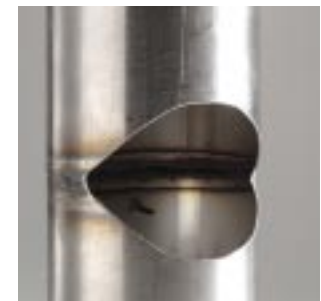
Unpurged Automatic Weld
